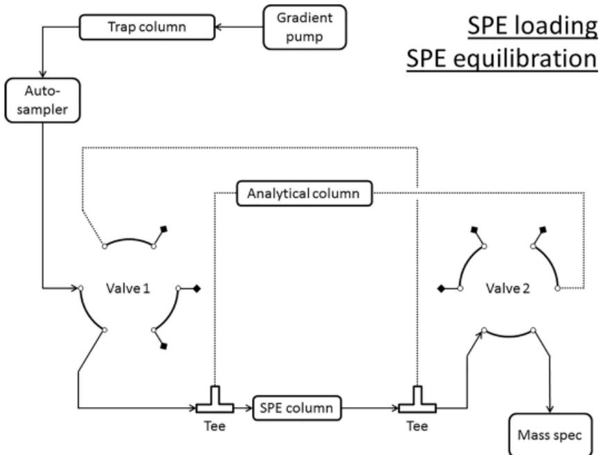
**Figure 4a** Flow chart of the online SPE HPLC system: SPE loading and equilibration.
