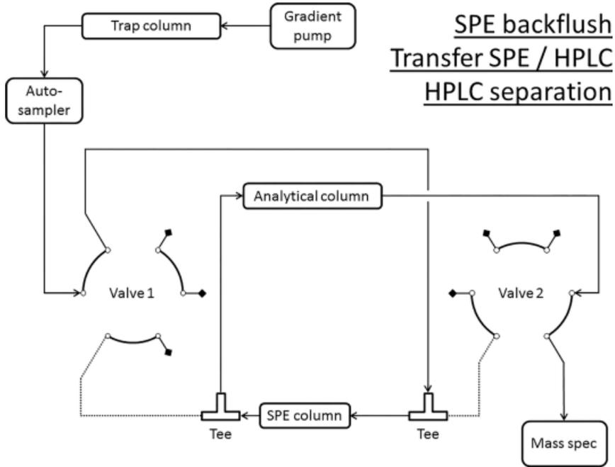
**Figure 4b** Flow chart of the online SPE HPLC system: SPE backflush, transfer and HPLC separation.
