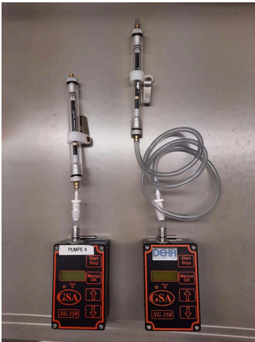
Fig. 1 Assembled sample carriers, at left for stationary measurements, at right for personal measurements. The assembly is made up of a sampling tube (type B/G) in a tube holder with a connecting tube and a sampling pump (SG350ex)
