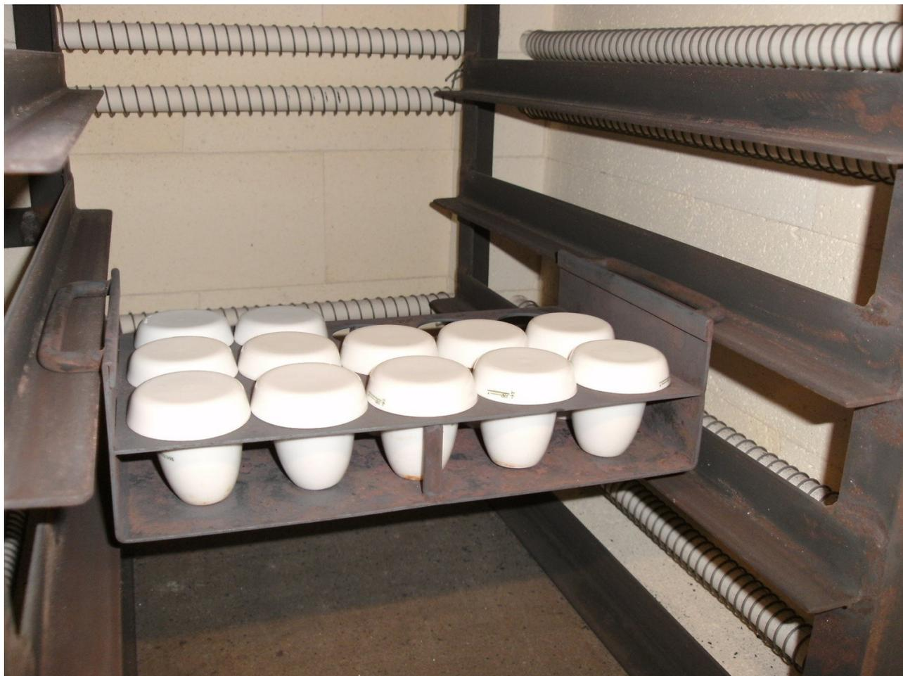
Fig. 2 Metal rack for insertion of the crucibles into the muffle furnace
