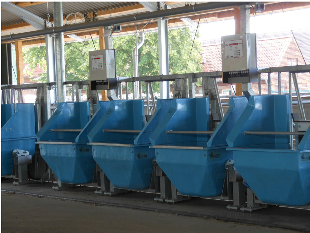
Figure 1: Automated individual feed intake measurement system (containing the digital display and feed bins)
