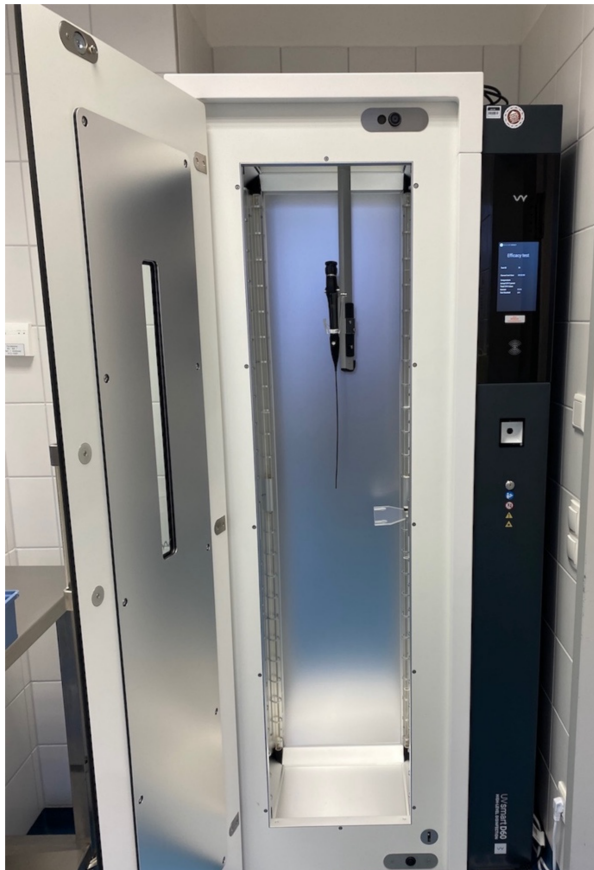
Figure 1: D60 UV disinfection system (UV Smart Technologies B.V., Rijswijk, Netherlands) with a thermolabile flexible otorhinolaryngological endoscope inside, as it is used in clinical routine.
