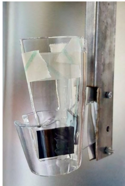
Figure 3: Thermoplastic elastomer (TPE 13(2)) samples, arranged in the D60 disinfection system hanger
