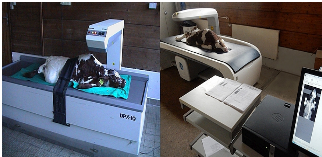
Figure 4: Calf positioned on a pencil beam DXA scanner (GE Lunar DPX-IQ) (left), and on a “narrow” fan beam scanner (GE Lunar iDXA) (right).
