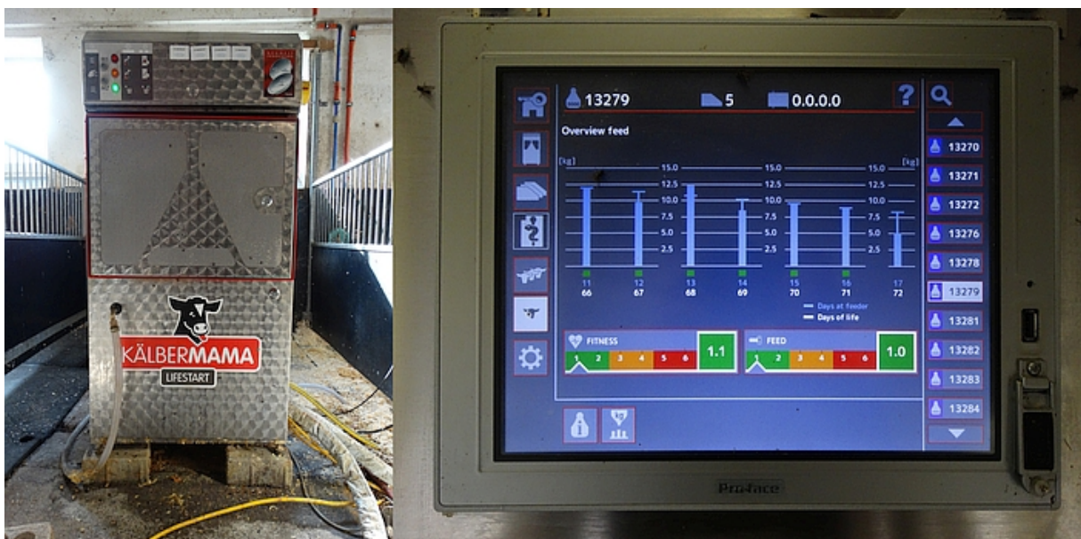
Figure 1: The left picture depicts an auto feeder system for rearing calves. The picture on the right shows the touchscreen, which displays calf management info: the amount of milk/MR the calf is drinking and alarms related to drinking behaviour.
