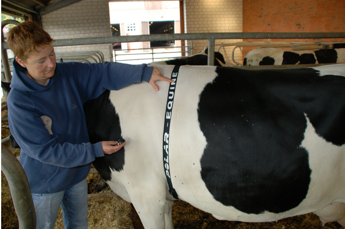
Figure 1: The polar electrode belt fixed on the animal with a staff member recording the HR data using the transmitter
