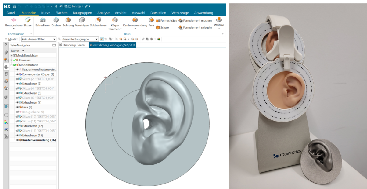
Figure 2: Design of the artificial ear canal, with the 3D-printed model to the right
